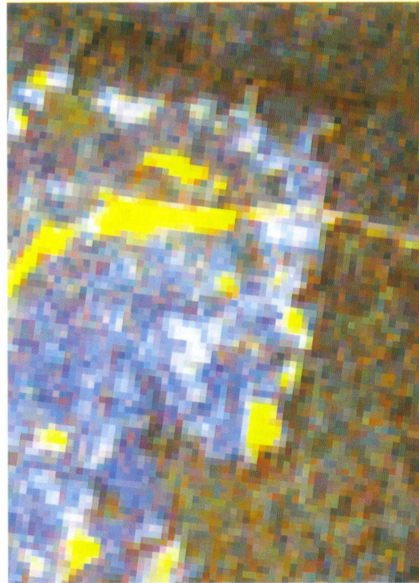
Fig. 12. Landsat image of the study village. Bands 7 (mid-infrared [ 2.08\text{-}2.35\ \mu\text{m} ]), 5, 4 are used in this scene. This combination makes the difference of the vegetations conspicuous.
